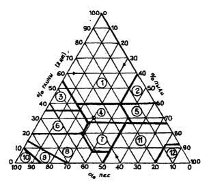
Fig. 1. The USDA textural triangle for classification of soil mixtures
