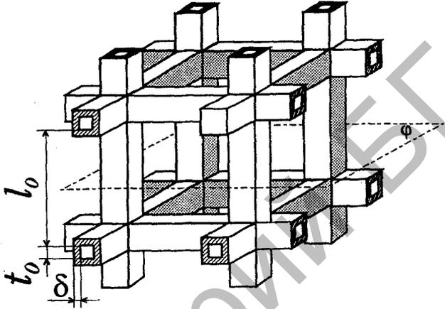
Fig. 4. Model of a foam structure
