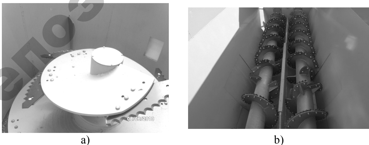
Fig. 8.7. Mixer–chopper feed: a) with a vertical cone–shaped screw b) with horizontal augers
