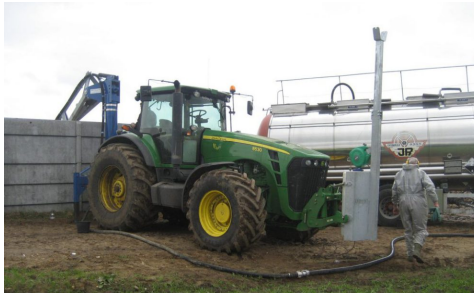
Figure 2. – OrumSemden’s “in storage” acidification system at work (farm in Denmark) Source: ORUM Co promotion material 2017
