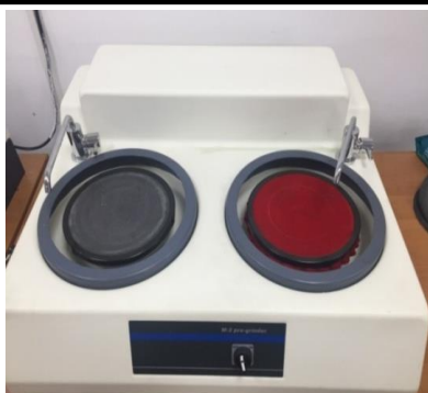
Figure 2 – Machine for preliminary grinding of metallographic specimens
