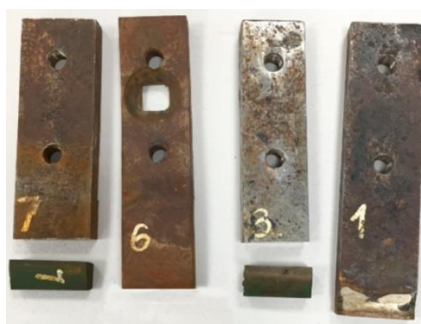
Sample 1 – clad with T590 carbide electrode, sample 3 – HFC-hardened, sample 6 – clad with CS-1 sormite, sample 7 – typical (factory) heat treatment method
