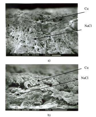
Fig. 6 Copper coating on the NaCl-CMC composition at various magnifications, x: a) × 150; ) × 800
