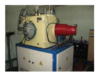
Fig.3 A vacuum machine HHB-6.6-U1 for the application of vacuum composite functional coatings
