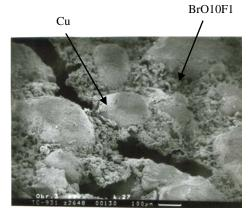
Fig. 9 Cracking at the fracture site of the experimental sample
