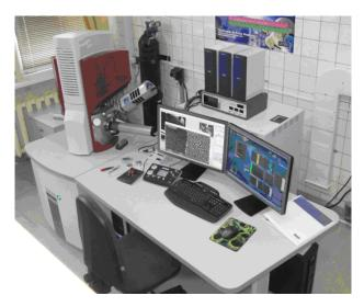
Fig. 2 A high-resolution scanning electron microscope "Mira-3" of Tescan company (Czech Republic)
