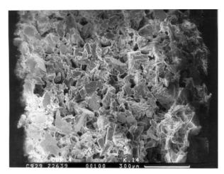
Fig. 4 The porous structure of NaCl-CMC
