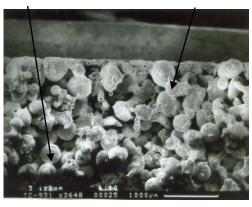
Fig. 8 Structure of a two-layer PPM, ×025
