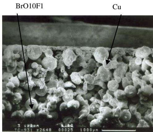
Fig. 8 Structure of a two-layer PPM,  $\times 025$
