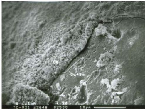
Fig. 12 The boundary line between the sputtered layer and the substrate particle at the site of brittle fracture
