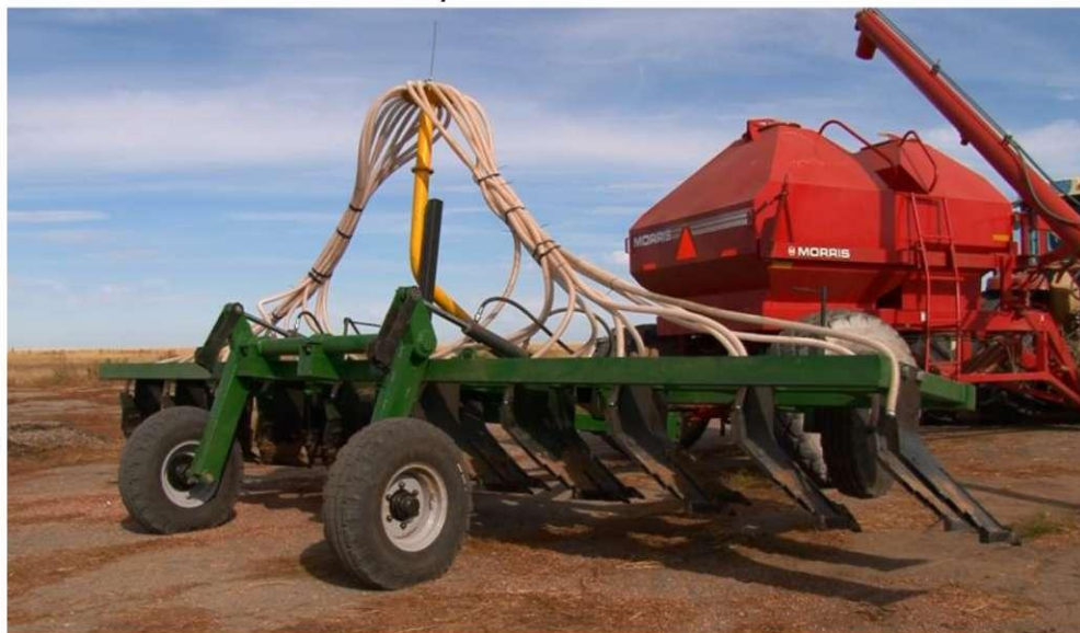
Figure 5 - A prototype of a chisel-fertilizer
