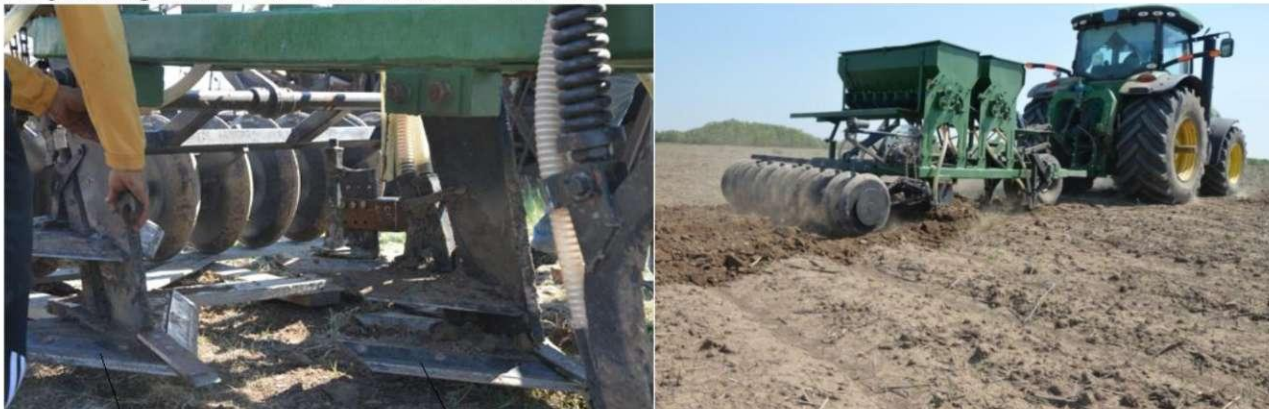
Figure 7 - A prototype blade plough-ripper-fertilizer
