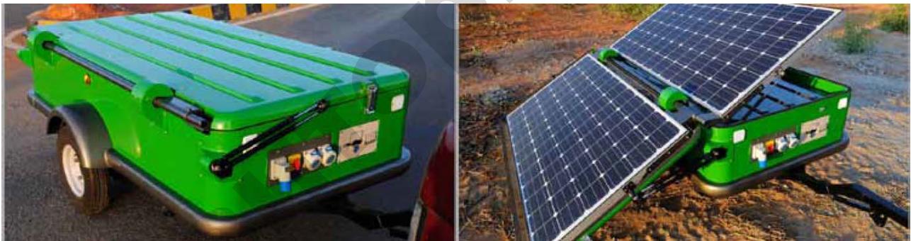
Figure 7.12. A mobile installation with a photoelectric converter to power self-contained devices in places with a limited power supply
