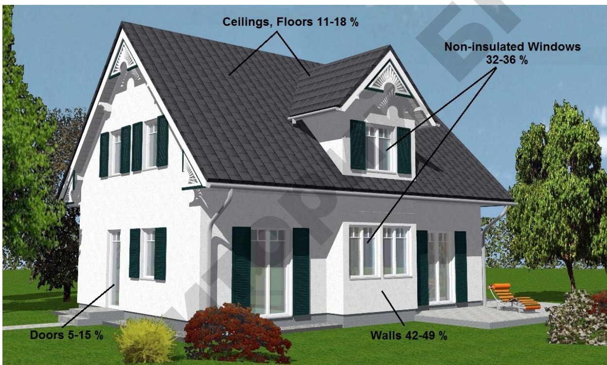
Figure 3.3. Heat energy losses due to the wallings of an individual dwelling house
