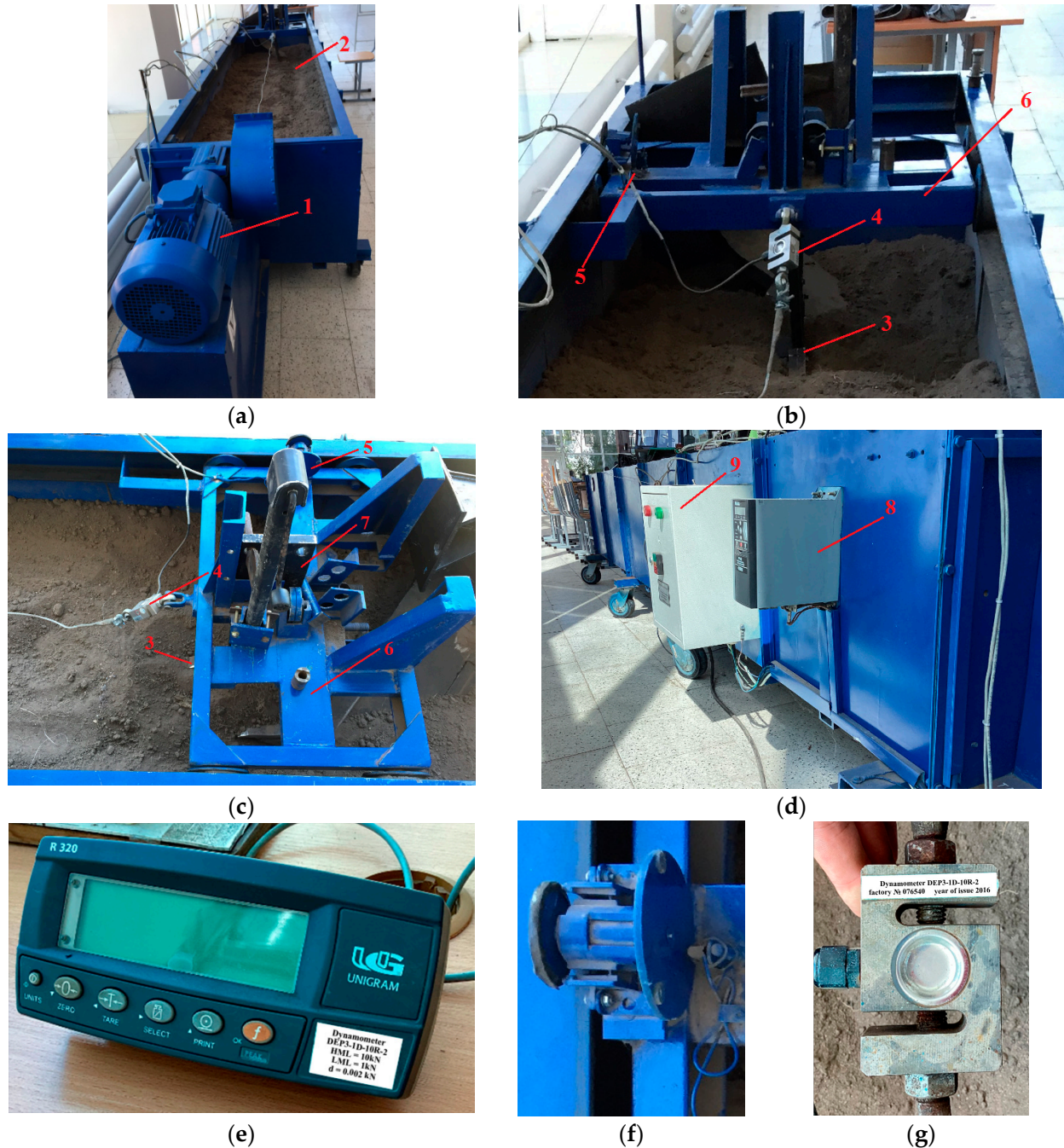
Figure 1. General view of the soil bin laboratory setup: (a) frontal view; (b) experimental working body in a soil bin; (c) top view; (d) side view; (e) indicator R320 (1); (f) velocity sensor; (g) dynamometer: (1) electric motor, (2) soil bin, (3) chisel, (4) dynamometer, (5) velocity sensor, (6) mounted truck, (7) working body shank; (8) vector frequency converter, (9) power board.
