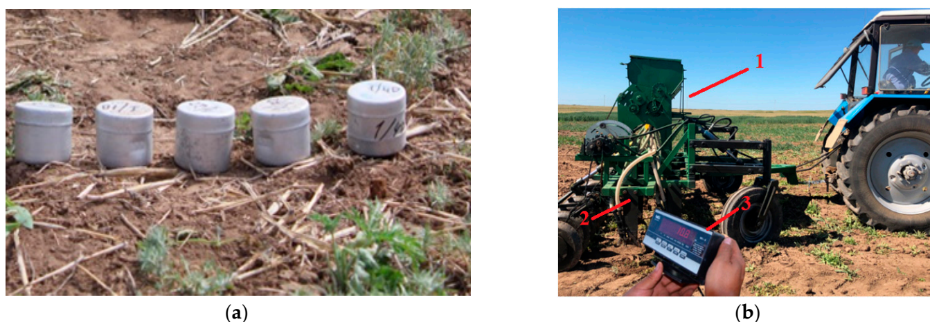
Figure 3. Determination of soil moisture and hardness: (a) bugs for moisture determination; (b) determination of the total traction force of the experimental grain–fertilizer–grass seeder: (1) experimental grain–fertilizer–grass seeder, (2) work body shank, (3) electronic dynamometer model DEP1-1D-50P-2.
