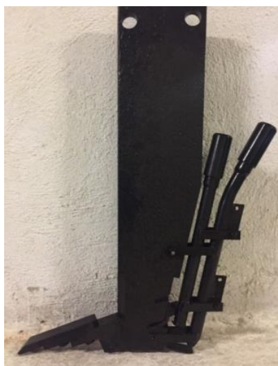
a) Experimental opener-splitter
