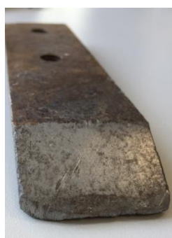
h) sample with thermally treated working surface according to factory technology
